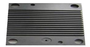
Bipolar Plates constitute an essential part of the FC and account for about the 35% of the overall cost and the 80% of the weight. Among their functions are: conducting electricity, transporting the gases that must react (hydrogen and oxygen) and eliminating the water produced. It should be noted that the various functional components of the cell, and the Bipolar Plates in particular, are not independent parts, but must be perfectly integrated and adapted to each other.
